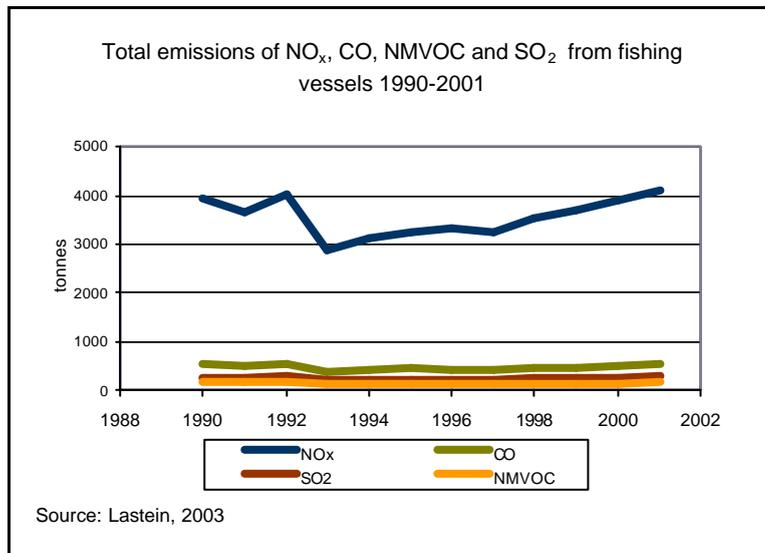
Figure 2.7: Total Emissions of No<sub>x</sub>, CO, NMVOC and SO<sub>2</sub>
